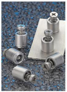
Panel fastener assemblies are used on enclosures where the screw must remain with the door or panel. Usually spring-loaded, these fasteners offer the advantages of ease of assembly and quick panel removal without loose screws. Photo courtesy PennEngineering
