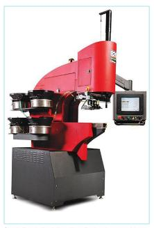
SingleTouch Part Handling Technology enables a press to insert up to four different self-clinching fasteners in a single handling of a part. Photo courtesy PennEngineering
