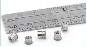
MSOFS flaring standoffs are manufactured from 300 series stainless steel and are offered in thread sizes #0-80, #2-56, and M1 to M2. They can be installed in panels from 0.008 to 0.012 inch thick. *Photo courtesy PennEngineering*
