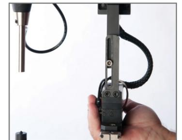
New T-bracket and shuttle with integrated connectors.
