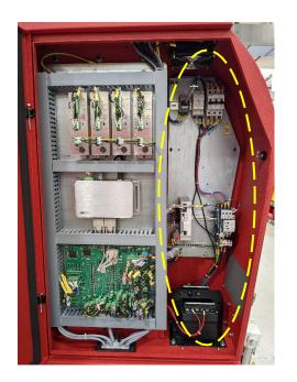
Risk of Electrical Shock: A high risk of electrical shock is present while working on the RIGHT HALF of the electrical cabinet.
