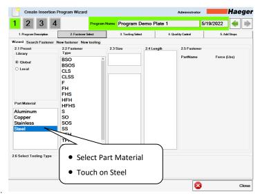
Part Material: Material of the work piece/panel (Not the fastener).
