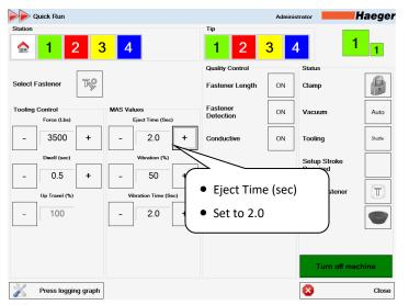
**Eject Time (Sec):** The Eject Time controls duration of the air blast which sends the fastener from your MAS 350 bowl to the automatic tooling at the work area. Adjust this time as needed for the fastener to properly reach the work area.
