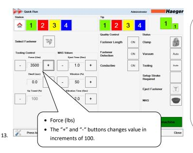
Force (lbs): Is the amount of force that will be applied during the hardware insertion cycle. The force can range from 800 pounds (3.6KN) to 16,000 pounds (71.2 KN). The 3300 lbs value displayed is derived from a manufacturers table of values however it can be adjusted by
