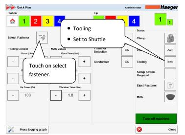
**Tooling:** This feature allows the operator to select the type of tooling to run in the selected station.
