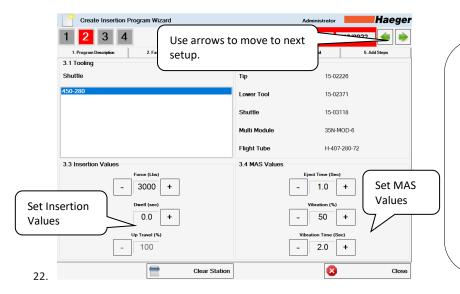
**Tooling:** Select correct tooling for current job
