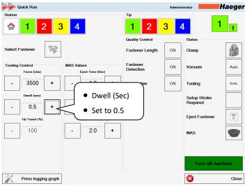
**Dwell (Sec):** Dwell is the length of time that the insertion force is applied. It can range from 0.0 seconds to 3.0 seconds. Setting the Dwell to 0.0 seconds will immediately return the ram upward after applying insertion force. A Dwell value greater than 0.0 seconds will keep the ram down, applying insertion force for that set amount of time.
