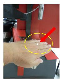
Risk of crushing: A high risk crushing hazard is created between the Punch and Anvil.
