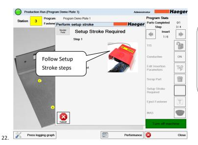
**Setup Stroke:** This feature sets up and records the fastener pickup point, fastener length, and insertion point. This only needs to be setup the first time for each station when running a program.
