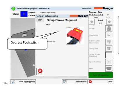
**Setup Stroke:** This feature sets up and records the fastener pickup point, fastener length, and insertion point. This only needs to be setup the first time for each station when running a program.
