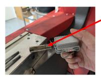
• 8<sup>th</sup>: Wipe off cylinder pin with dry clean cloth and apply a **thin film** of lithium grease around the pin.
