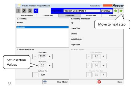
**Tooling:** Select correct tooling for current job
