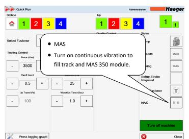
Modular Auto Feed System (MAS): This feature allows the operator to either run the MAS 350 at a continuous vibration or an intermittent vibration.
