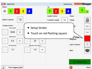
Setup Stroke : This feature sets up and records certain values for the current auto-tooling station and project run. This must be completed at the beginning of each Quick Run and each station.
