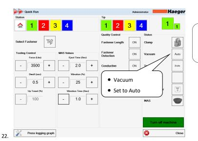
**Vacuum:** This feature allows the operator to switch the vacuum system ON or OFF on the vacuum punch.
