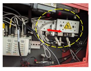
Risk of pinching: A medium risk pinching hazard during maintenance of adjusting nuts on Lower Tool Indexing assembly.
