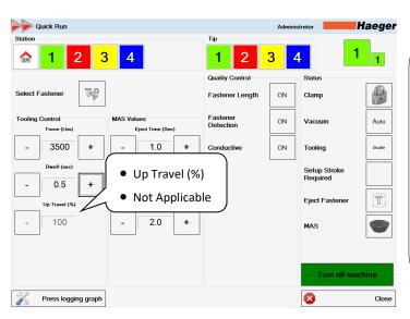
Up Travel (%): The Up Travel value controls the Up Position of the ram. This is the upward position the ram returns to after applying insertion force. The Up value is measured as a percentage of the total cylinder stroke. It will vary depending on the lengths of the Upper and Lower Tools.
