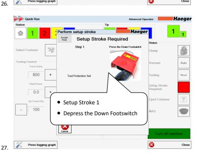
Setup Stroke Step 1 - Station
