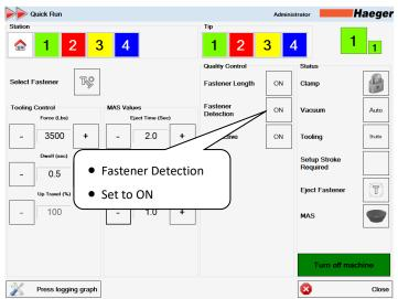
Fastener Detection: This will instruct the machine to perform detection of a fastener at the fastener pickup point of the Shuttle Tooling Jaws. The Fastener Detection can be activated or deactivated by touching the Fastener Length ON/OFF button.
