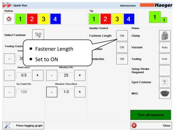
Fastener Length: This will instruct the machine to verify fastener length when contact with the anvil is detected. This can be activated or deactivated by touching the Fastener Length ON/OFF button.
