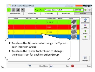
A Tip or Lower Tool from a different station may be used if desired.
