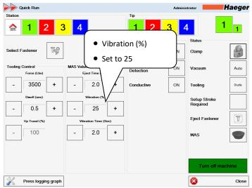
**Vibration (%):** Vibration controls the MAS 350 bowl vibration speed. This determines how fast the hardware travels up the spiral track to reach the Multi Module.
