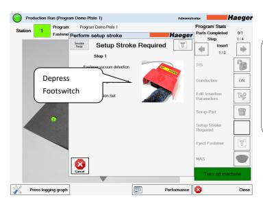
**Setup Stroke:** This feature sets up and records the fastener pickup point, fastener length, and insertion point. This only needs to be setup the first time for each station when running a program.
