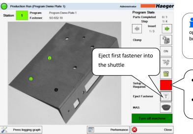
**Eject Fastener:** This feature allows the operator to eject a fastener from the MAS bowl to the automatic tooling system.
