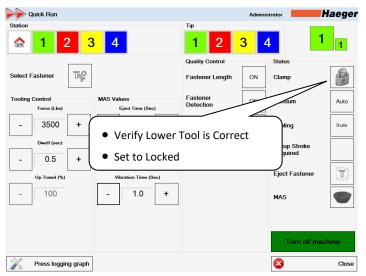
**Clamp:** This feature allows for the operator to lock or unlock the anvil, allowing it to be removed and replaced manually.
