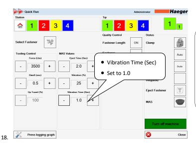
Vibration Time (Sec): Vibration Time controls the duration that the MAS 350 bowl will vibrate after a fastener has been ejected. Adjust the vibration time as needed to keep a full track of hardware.
