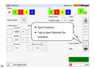
**Eject Fastener:** This feature allows the operator to eject a fastener from the MAS bowl to the work area.
