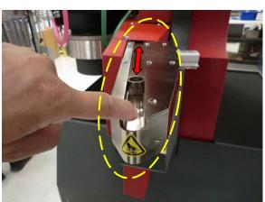
Risk of pinching: A medium risk of pinching hazard created by the Upper Tool Changer moving back and forth while changing Vacuum Tips and receiving fasteners.
