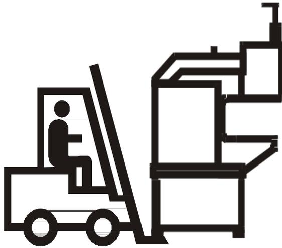
**Always position the forklift to the rear of the machine.**
