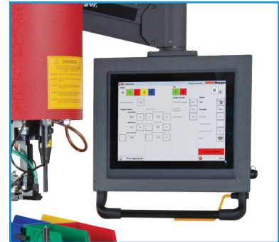
Operator control pendant adjustable in 6 directions.
