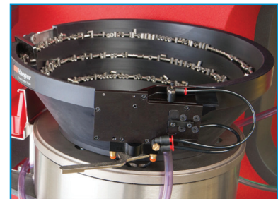
MAS 350 - new modular autofeed system.
