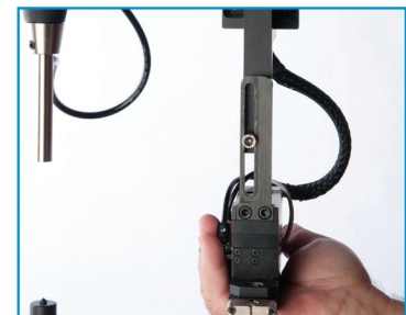
New T-bracket and shuttle with integrated connectors.
