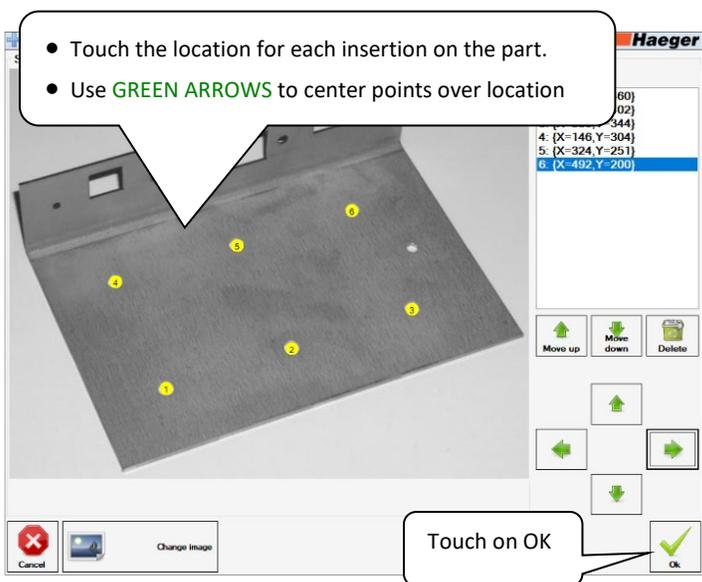
**Select Points:** Add Insertion Points to the image by tapping the desired location on the image. Use the four direction arrows on screen to fine-tune and center the point.
