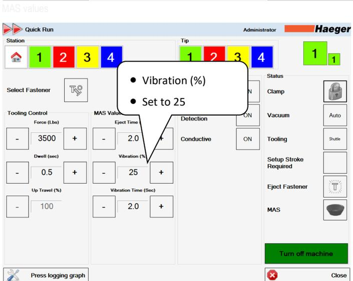
**Vibration (%):** Vibration controls the MAS 350 bowl vibration speed. This determines how fast the hardware travels up the spiral track to reach the Multi Module.
