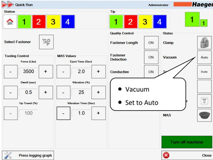
**Vacuum:** This feature allows the operator to switch the vacuum system ON or OFF on the vacuum punch.
