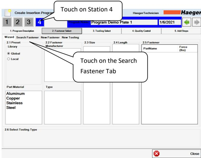
Speed up the programming steps by using Search Fastener in lieu of the wizard to program Station 4.
