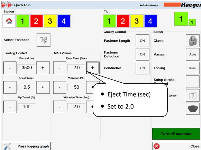
**Eject Time (Sec):** The Eject Time controls the duration of the air blast which sends the fastener from your MAS 350 bowl to the automatic tooling at the work area. Adjust this time as needed for the fastener to properly reach the work area.
