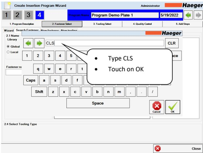
**i** To go directly to the desired fastener, type in the fastener's identification number. (ex. CLS-M10-1)
