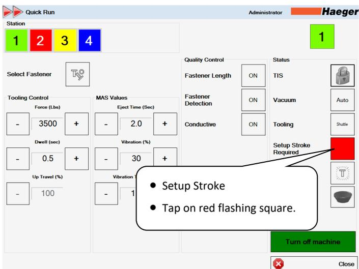
**Setup Stroke** ■: This feature sets up and records certain values for each station and project run. This must be completed at the beginning of each Quick Run.
