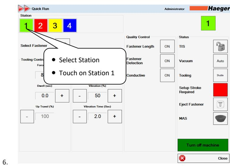
Station: Station **1** is a high volume, **Automatic** insertion station working in conjunction with the Modular Automated Feed System (MAS).
