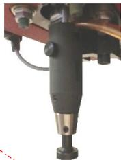
It is recommended to inspect the upper tool holder and its contacts weekly or more frequently based on usage.
