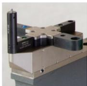
It is recommended to inspect the TIS-3 and its contacts weekly or more frequently based on usage.
