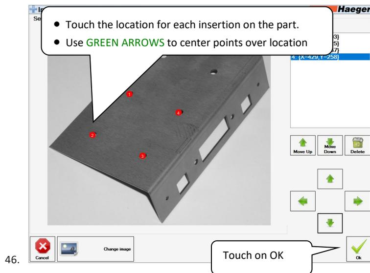
**Select Points:** Add Insertion Points to the image by tapping the desired location on the image. Use the four direction arrows on screen to fine-tune and center the point.
