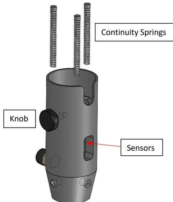
If the Upper Tool Holder moves up .015 in/0.4 mm to 0.02 in/0.5 mm, the Safety Sensors will be triggered, and the ram will be raised. Should only one of the Sensors be triggered, the ram will be raised.
