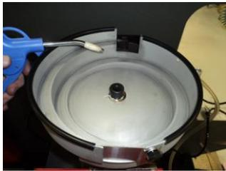
2<sup>nd</sup>: Use dry compressed air to blow out debris.
