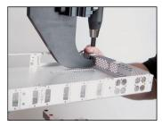
Manual tooling J-Frame is used for small boxes and short reverse flanges.
