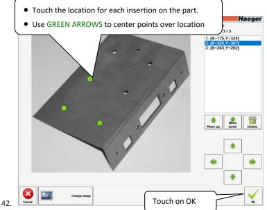
**Select Points:** Add Insertion Points to the image by tapping the desired location on the image. Use the four direction arrows on screen to fine-tune and center the point.
