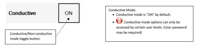
In **Non-Conductive Mode**, the machine will lower the ram until contact is made with the work piece then stop. The Down Footswitch must then be released. **Depress the Down Footswitch a second time, to exert force.** The ram will return to its Up position after. Once the upward travel begins, release the Down Footswitch.
