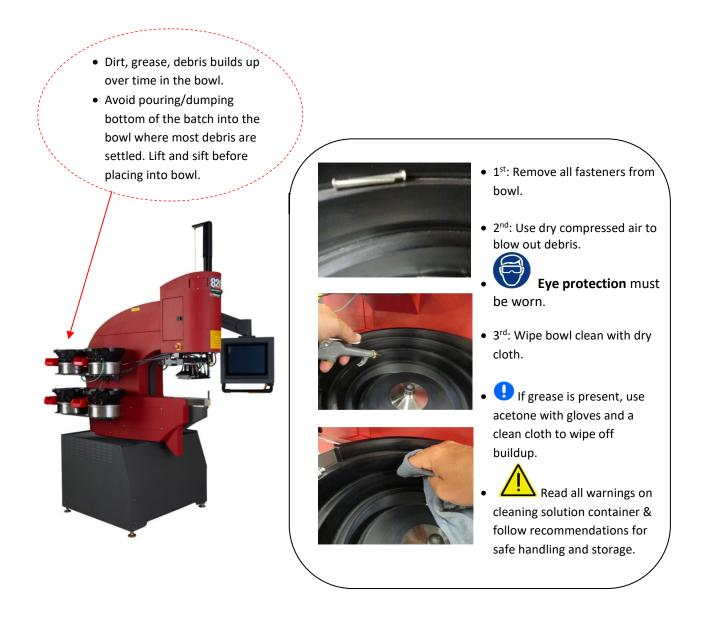
DO NOT use rubbing alcohol, WD-40, diesel, gas, etc., to clean MAS 350 composite bowls!
