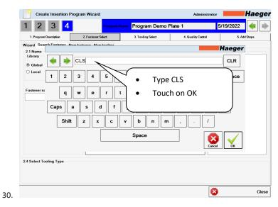
To go directly to the desired fastener, type in the fastener's identification number. (ex. CLS-M10-1)
