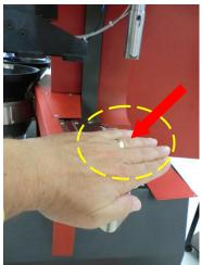
Do not operate this machine while wearing any metal objects (i.e., rings, watches, bracelets, etc.) that may come into contact with the Punch, Anvil, or work piece.
