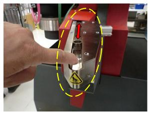
**Risk of pinching:** A medium risk of pinching hazard created by the Lower Tool Slide moving back and forth while exchanging lower tools.
