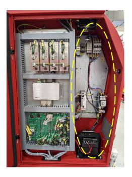
**Risk of Electrical Shock:** A high risk of electrical shock is present while working on the **RIGHT HALF** of the electrical cabinet.
