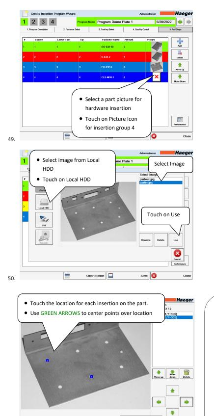
**Select Points:** Add Insertion Points to the image by tapping the desired location on the image. Use the four direction arrows on screen to fine-tune and center the point.
