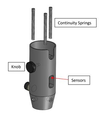
If the Upper Tool Holder moves up .015 in/0.4 mm to 0.02 in/0.5 mm, the Safety Sensors will be triggered, and the ram will be raised. Should only one of the Sensors be triggered, the ram will be raised.
