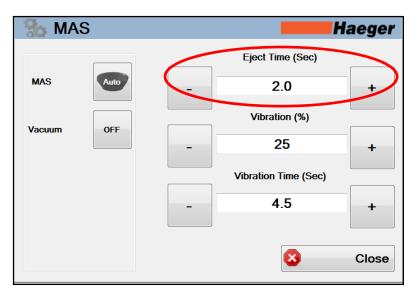
Eject Time (sec): The Eject Time controls how long of an air blast the fastener will receive when traveling through the flight tube to the shuttle jaws. The Eject Time can range from 0 to 20 seconds. This value can be increased or decreased by touching the + or – symbols on either side of the value or by touching the value box and typing in a new value.
