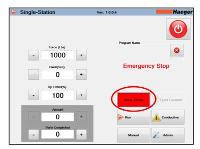
**Setting the TPS:** The Tool Protection System (TPS) allows for the operator to do a first stroke setup of the tooling. This is done to ensure the safety of the operator and the tooling by allowing only the correct length of fastener to be inserted.
