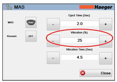
Vibration (%): The Vibration controls the amount of vibration needed to move the fasteners through the MAS bowl. This value can be increased or decreased by touching the + or – symbols on either side of the value or by touching the value box and typing in a new value.
