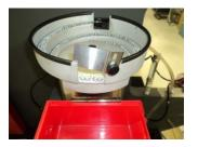
Dirt, grease, and debris builds up over time in the bowl.
