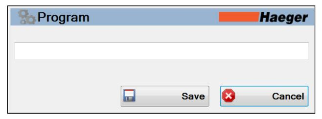
**Save:** The Save screen appears after selecting "Save" in the Administration screen. The Save screen allows the operator to save the settings that are currently in use for each station. By pressing on the white label, a touch type keypad allows for the naming of the program.
