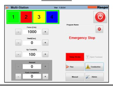
**Multi-Station**: Multi-Station is an option that allows the operator to insert more than one fastener in a program. The maximum number of fasteners in an individual program is 4. Each station can be selected by pressing on the color coded numbers at the top of the screen. \*Note: only station 1 can be used for manual tooling, Shuttle style tooling and ABFT style tooling.
