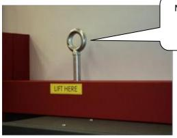
Machine is HEAVY in REAR and will tilt back when lifted with strap
