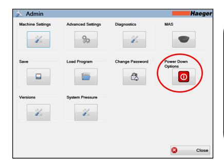
**Power Down Options:** Select the Power Down Options button to shut down the machine.
