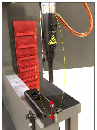
Risk of crushing: A high risk crushing hazard is created by the Upper Tool and Lower Tooling.
