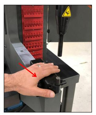
Do not operate this machine while wearing any metal objects (i.e., rings, watches, bracelets, etc.) that may come into contact with the *Upper Tool, Lower Tool* or work piece.
