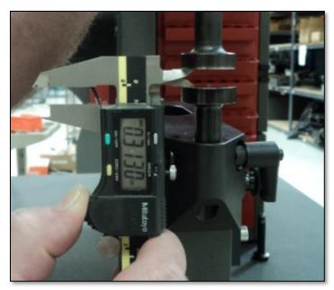
a. If this dimension is less than 1/4 in. /6 mm, the Safety System has failed!
