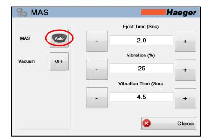
MAS Auto/MAS On: This button allows the operator to run the MAS bowl full time or intermittently.
