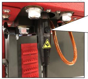
Important: If this thumb screw is lost, DO NOT replace it with just any length 5mm screw. Using too long of a screw will damage the Ram Adapter.
