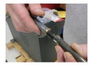
• 3<sup>rd</sup>: Rinse inside of tube with Denatured Alcohol and air dry.
